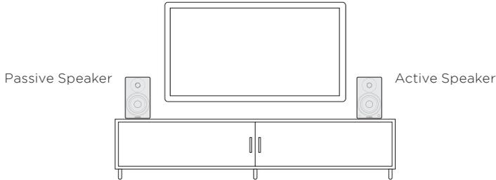
**NOTE:** If placing the speakers in a cabinet or on a shelf, position the front of the speakers as close as possible to the front edge of the shelf for optimum audio performance.
