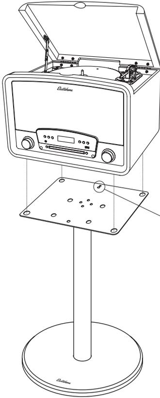
When lowering the RR75 onto stand, place the feet into the holes to ensure stability.
