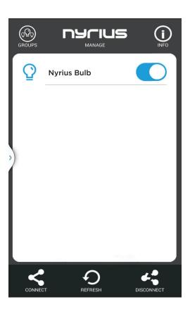
Control a bulb independently or add more Smart Bulbs to create zones so you can control specific areas in your home. You will see a list of smart bulbs within Bluetooth range that are available to control. If you do not see the smart bulb you wish to control in the manage screen, press refresh and ensure you are within Bluetooth range. Up to 8 Smart Bulbs can be seen on the mange screen at one time.
