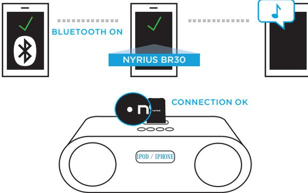
\* NYRIUS LED FLASHES WHEN SEARCHING FOR SIGNAL. LED DIMS AFTER 60 SECONDS UNTIL A SIGNAL IS RECEIVED.
