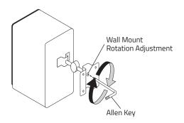
**4.** Use the wall mount rotation adjustment to rotate the speaker mount to the desired position.
