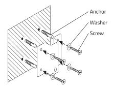
**7.** Place Wall Bracket in place and use washers and screws to secure. If installing in concrete or drywall, insert anchors into predrilled holes before securing.
