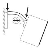
**8.** Once the speaker is mounted, install the steel safety cable through both safety cable holes.
