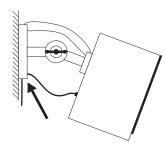
**9.** When connecting the speaker wire feed it through the wire hole for easy wire management.
