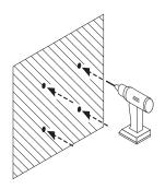
**6.** If installing in concrete or drywall, drill holes to match the size of the included mounting hardware.
